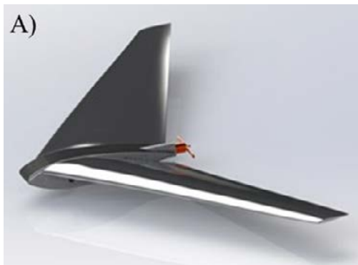
A) Rendering of an UAV with a 12 foot wingspan designed for fabrication and flight to demonstrate the effectiveness of the Prandtl-D wing
