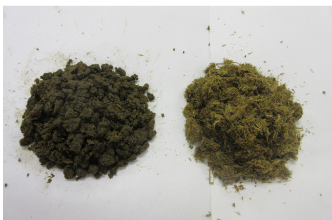
Figure 2. Centrifuge-separated solids (left) and screen-separated solids (right).
